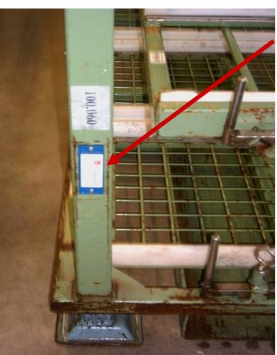
RTI's are equipped with two transponders
