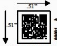
Figure 5. QR Code Symbol with .020" Element Size
